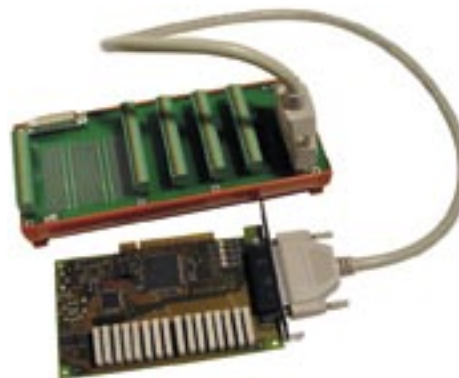
ME630 PCI Card and ME-ABD78MSH Heavy Duty Terminal Box with Spring Clips
